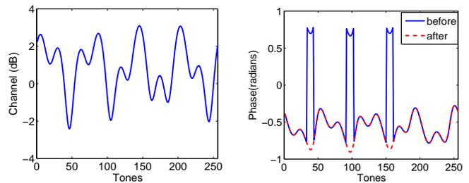
Fig. 2. Amplitude and phase channel estimates before phase unwrapping and after phase unwrapping with WiMAX parameters and QPSK constellation on a SUI-1 channel model
