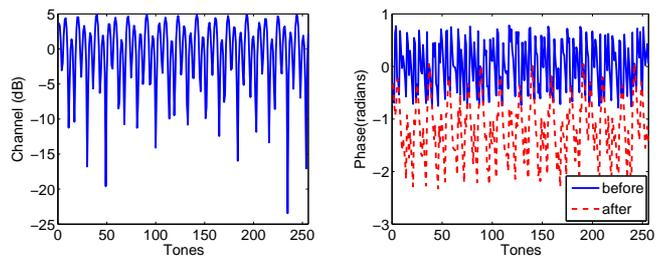
Fig. 3. Amplitude and phase channel estimates before phase unwrapping and after phase unwrapping with WiMAX parameters and QPSK constellation on a SUI-4 channel model
