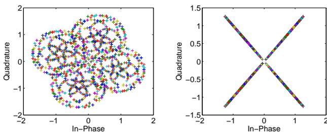
Fig. 1. Frequency domain demodulated CP-OFDM symbol before and after phase offset correction by modulation stripping with WiMAX parameters and QPSK constellation on a SUI-1 channel model
