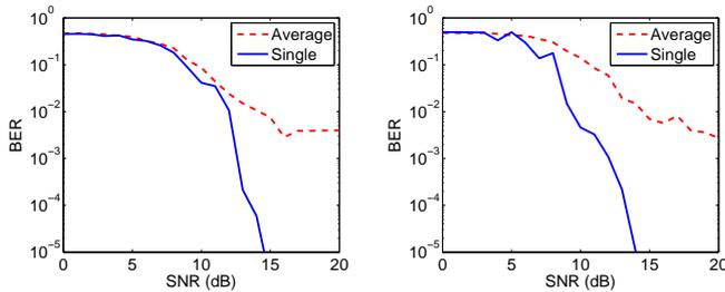
Fig. 4. BER curves for blind demodulation of CP-OFDM (left) and ZP-OFDM (right) transmission
